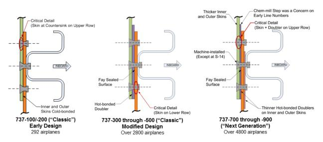
Fig. 7 – Boeing 737 fuselage skin lap splice design evolution.
