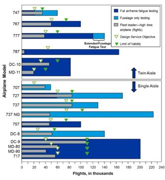
Fig. 16 – Boeing fleet data (as of May 2016) relative to DSO and full-scale fatigue test for twin aisle and single aisle-category airplanes.
