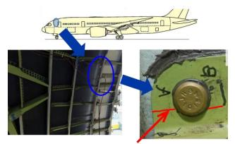
Crack highlighted for clarity
