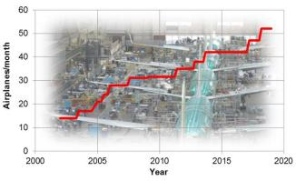
*Fig.* 36 – *Production rate forecast through 2018 (left) for the Boeing 737 NG and MAX.*
