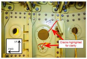
Fig. 19 – Example of a 787 full-scale fatigue test crack finding. Cracked satellite holes in the left and right (depicted here) side-of-body ribs immediately forward of the rear spar, found at the 132,000-flight inspection. This cracking was deemed acceptable for continuing cycling with increased surveillance.
