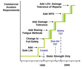
*Fig.* 2 – *Evolution of design requirements for commercial transports, and some of the events that shaped them.*
