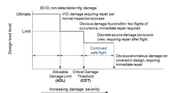
*Fig.* 25 – *Design load dependence on damage severity* (*adapted from* [22]).
