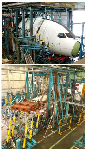
Fig. 32 – Boeing 787 full-scale fatigue test examples: Top: Section 41 (forward fuselage). Bottom: Center wing and outboard wing stub box.
