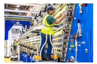
Fig. 37 – The 737 PAL wing assembly system. Automating the process of assembling the 737 wing panels is expected to reduce flow time and improve safety and quality.
