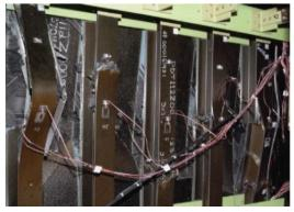
Fig. 30 – Example of configured element testing of composites (In the photo: Residual strength testing of stiffened panel with BVID).
