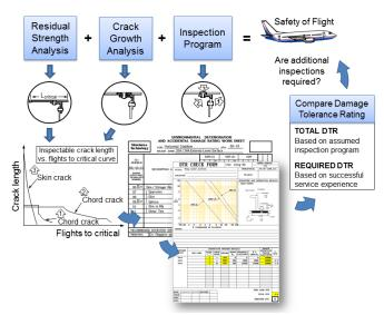
*Fig.* 10 – *Fundamental elements of the Boeing damage tolerance analysis method.*
