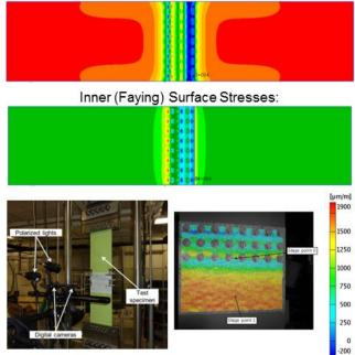
Fig. 41 – Fuselage lap splice analysis and laboratoryscale validation using optical DIC.
