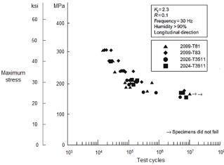
Fig. 34 – Typical constant-stress amplitude fatigue test data for notched aluminum (2024-T3511) and aluminumlithium extrusions (reproduced from [27]).
