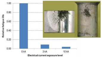
Fig. 29 – (Inset) Typical pitting and resulting fatigue crack resulting from a 10 kA per fastener step current through a hybrid CFRP-aluminum joint, standard titanium ¼-inch (6.4 mm) lockbolt installed in clearance and matching pin location. (Plot) CFRP-aluminum joint tests, standard titanium lockbolts installed in clearance [25].
