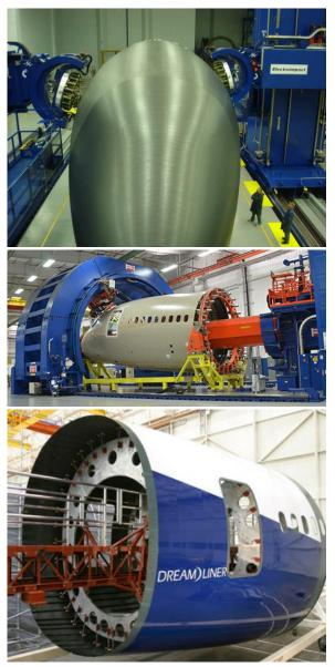
Fig. 22 – Large-scale composite structure manufacturing development for the Boeing 787 program. Numerous fuselage test barrels were constructed at Boeing and at 787 Partner facilities. The first composite fuselage section (bottom) was unveiled in January 2005.
