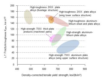
Fig. 33 – Fracture and strength properties of aerospace aluminum and third-generation aluminum-lithium alloys (Boeing data).
