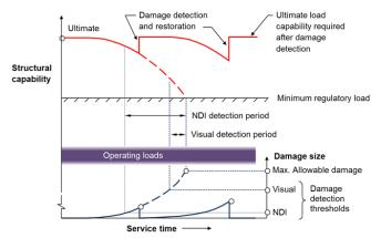
*Fig.* 9 – *Damage evolution, detection, and repair as a function of service time in damage tolerant structure.*
