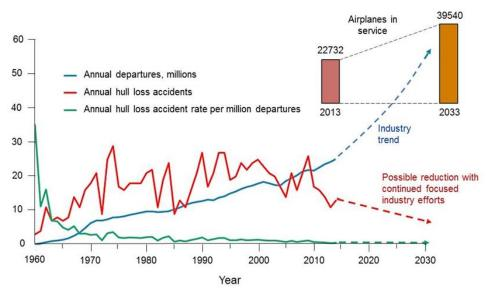
Fig. 1 – Annual hull loss accident totals and rates for the worldwide commercial jet fleet [6].
