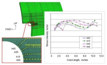
Fig. 43 – Boeing 747 Passenger door cutout crack growth analysis.
