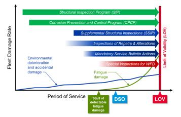
Fig. 15 – Strategies for ensuring fleet safety in the presence of fatigue, environmental deterioration, and accidental damage.
