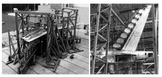
*Fig.* 24 – *Boeing* 777-200 *composite horizontal stabilizer and vertical fin full-scale fatigue tests (1993-94).*
