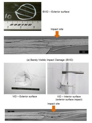
(b) Visible Impact Damage (VID) Fig. 27 – Typical damage: (a) BVID vs. (b) VID (from [23]).
