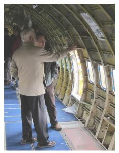
*Fig.* 44 – *Retired Boeing* 737 *fuselage training aid.*
