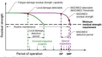
Fig. 12 – WFD typical implementation schematic.
