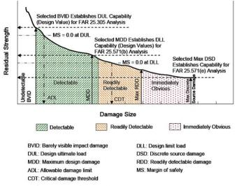
Fig. 26 – Design damage limits for composite structure.
