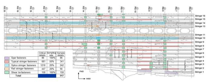
Fig. 20 – Boeing 777 full-scale fatigue test teardown activities on the outboard wing lower surface.
