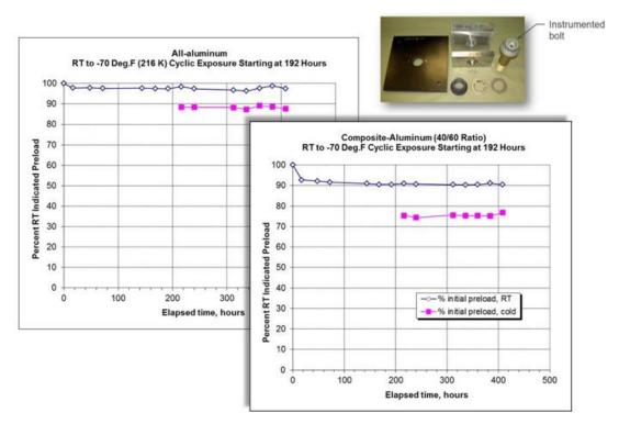
Fig. 28 – Half-inch (12.7 mm) nickel alloy 718 bolts in faying surface-sealed aluminum and hybrid joints aged at ambient temperature, then cycled cold [25].
