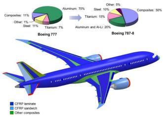
Fig. 21 – Boeing 787 Composite materials usage.
