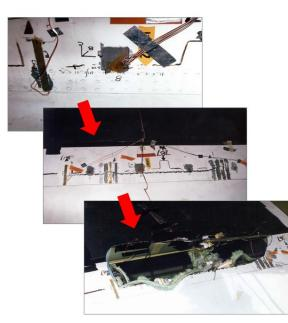
Fig. 11 – The classic WFD stages on a fuselage skin lap splice: Crack nucleation -> Coalescence -> Flapping.
