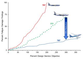
*Fig.* 17 – *Comparison of findings from the 767, 777 and 787 major airframe fatigue tests.*
