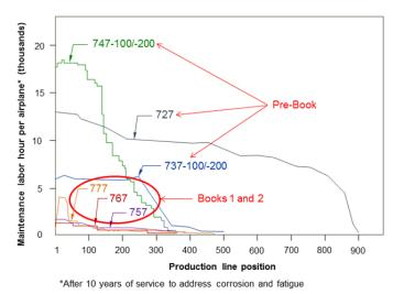
*Fig.* 6 – *Impact of new design and analysis practices on fleet maintenance hours.*
