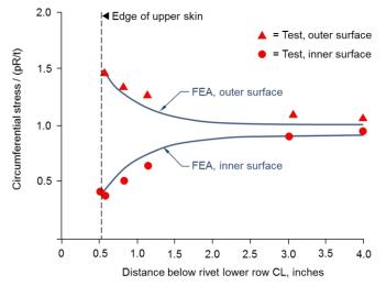
Fig. 42 – Finite element model correlation with ground pressurization test measurements on a Boeing 747 lower fuselage skin, below a longitudinal lap splice at mid-bay.
