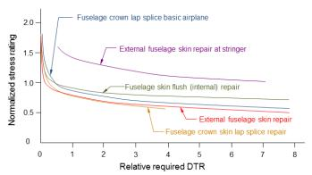
Fig. 14 – Normalized Stress Rating versus the multiple of required DTR for D/4C surveillance inspection for Pressure Critical Structure (reproduced from Ref. [14]).
