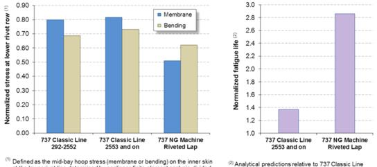
at the lower rivet line determined by nonlinear finite element analysis divided by pR/t, p = Operating pressure, R = Fuselage radius, t = Basic skin gage.
