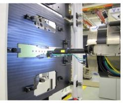
*Fig.* 38 – *Fatigue test specimen being assembled in a production 737 PAL gantry system.*
