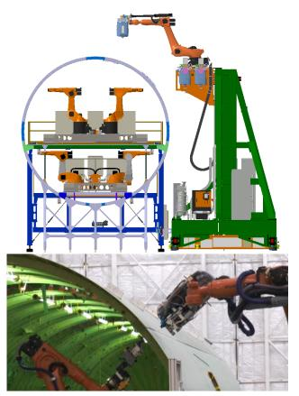
Fig. 39 – The Boeing 777 FAUB fuselage assembly process.
