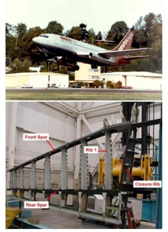
*Fig.* 23 – *Boeing* 737 *composite horizontal stabilizer technology demonstrator.*
